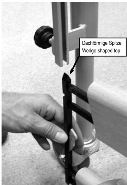
☞ Now place the 8 cm wide side rail beam [7] onto the top pair of metal plugs on the end board, head section, and let the other end of the side rail beams lie on the floor.
